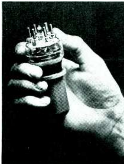
Full output of 1800 watts is available up to 150 Mc in the GL-8002 (left), up to 120 Mc in the air-cooled version
